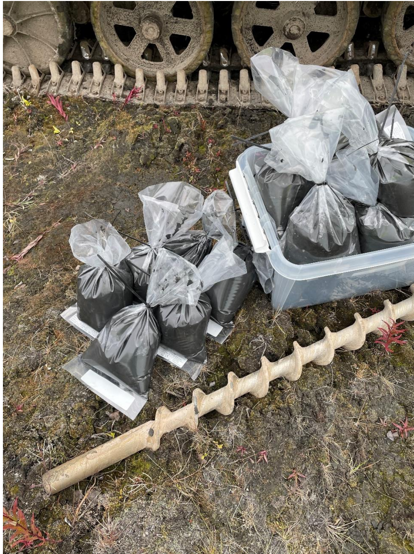
Figure 6. The samples were stored in plastic bags, closed with zip tie. The sample information was included with each sample.
