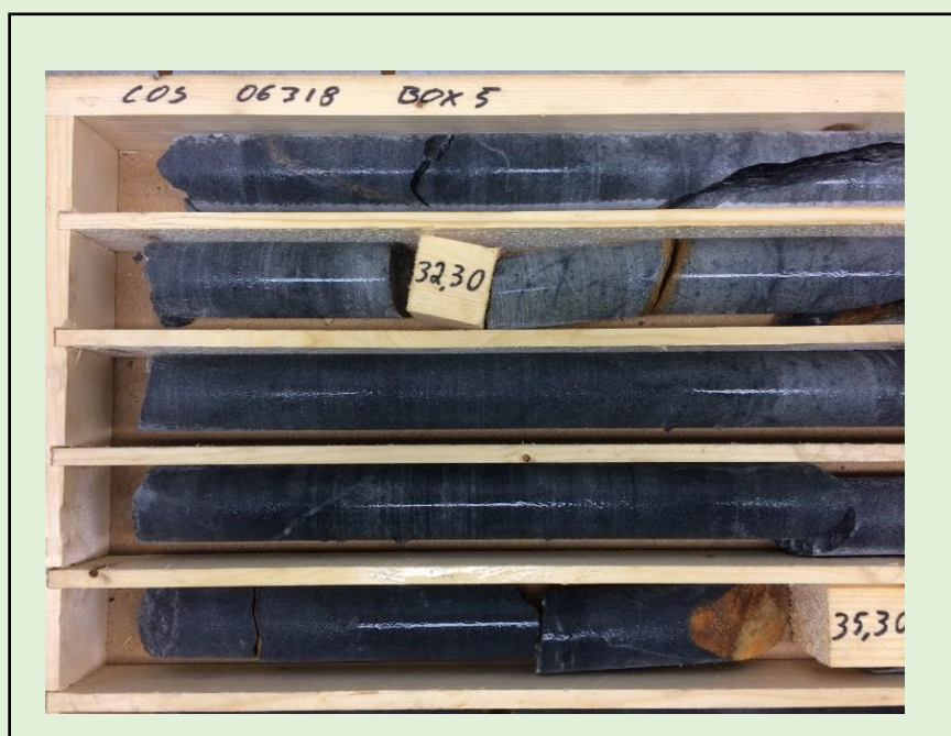
Figure 5: Hydrothermally altered core characterized by grey-green colour and relict sedimentary features.
